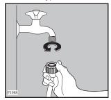
The inlet hose must not be lengthened. If it is too short and you do not wish to move the tap, you will have to purchase a new, longer hose specially designed for this type of use.
